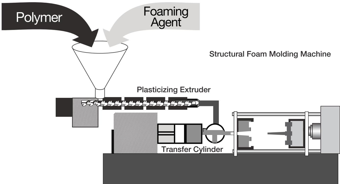
Typically, low-pressure structural foam molding machines designed for foam molding, are equipped with a plasticizing extruder and a separate accumulator cylinder for quicker injection.
