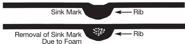
Injection molded parts which have been produced with chemical foaming agents are characterized by a mat surface. Glossy surfaces can only be achieved in special cases with small amounts of foaming agents. Bergen International has developed a special grade, Foamazol™ 62 that allows molders to eliminate sink marks without the swirled surfaces associated with foam-molded parts.
