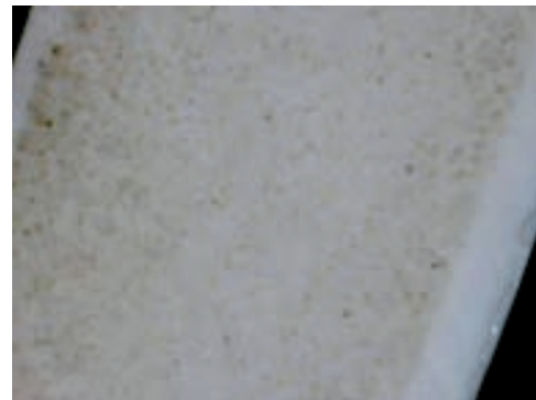
50x Magnification of Bergen's Cell Structure with XO-468 in PVC Pipe
