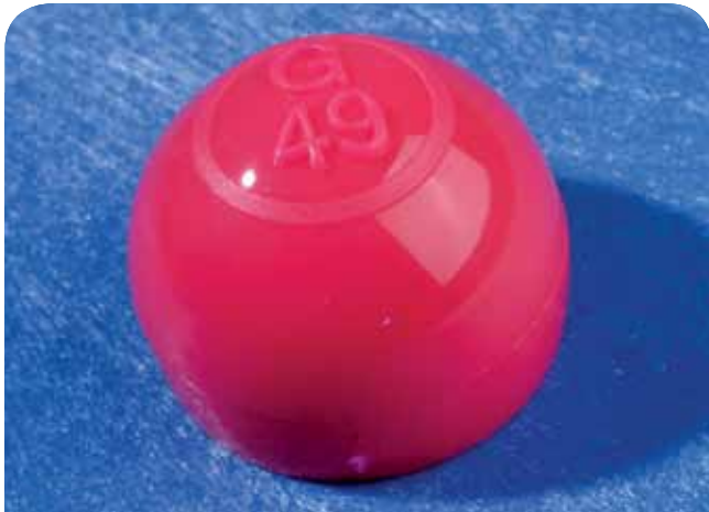
Class A surface with no swirl or sink marks.
