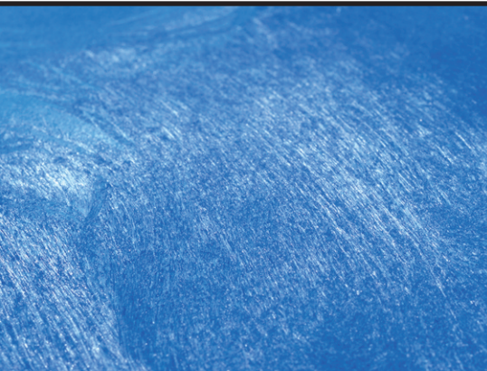
Swirled surface on plastic part in application where surface appearance is not critical
